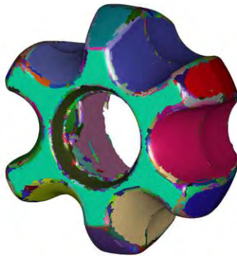
Fig. 2. Dihedral segmentation produces over-segmentation due to surface imperfections and surface blends
