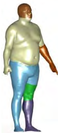
Fig. 18. Non-parameterizable segmentation of an organic mesh with our algorithm. Human mesh from the Princeton benchmark [41].
