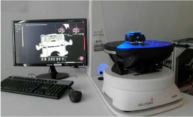
Fig. 8. Acquisition of 3D point cloud data through an optical 3D scanner
