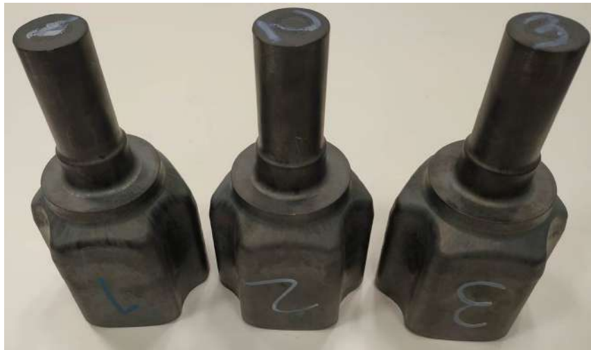
Figure IV-E.2.11: Cold workpieces used to run the ANOVA R&R test. The three workpieces share the same CAD reference.
