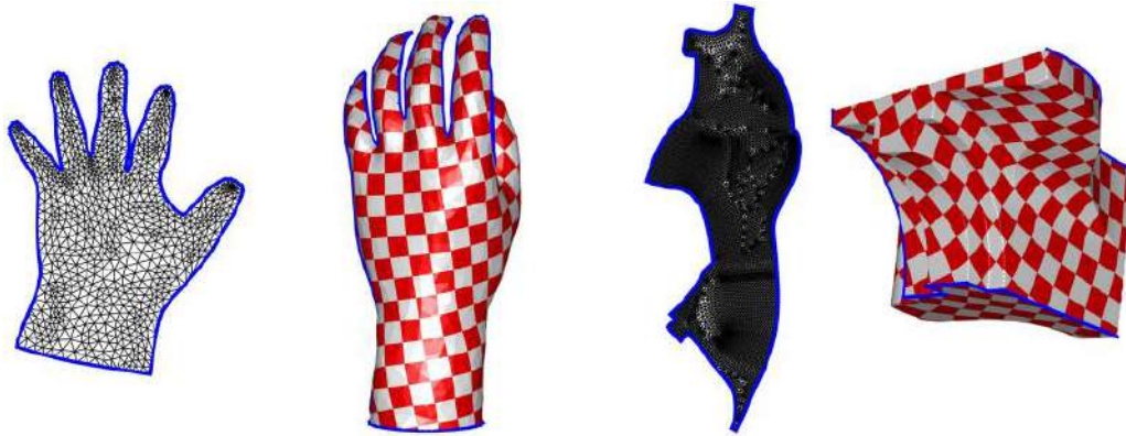
(a) Sliced-Glove bijective parameterization and texture map. (b) Fandisk bijective parameterization and texture map.
