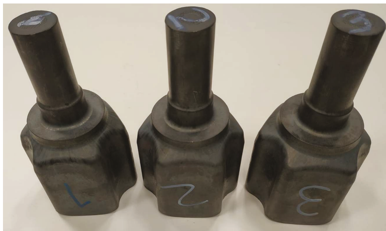
Figure 11. Cold workpieces used to run the ANOVA R&R test. The three workpieces share the same CAD reference.
