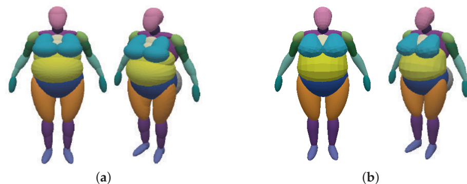
Figure 7. Mannequin approximated with cushions and ellipsoids. Ellipsoid mannequin (a) for comparison. Cushions computed according to Figure 5. Small chubby mannequin (see Section 3.3) as (a) Ellipsoid-based Mannequin and (b) Cushion-based Mannequin.
