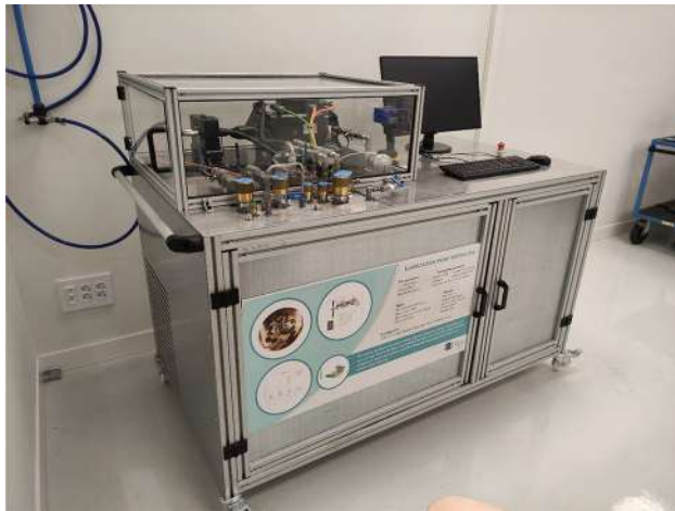
Fig. 14 Dedicated Gerotor testbed
