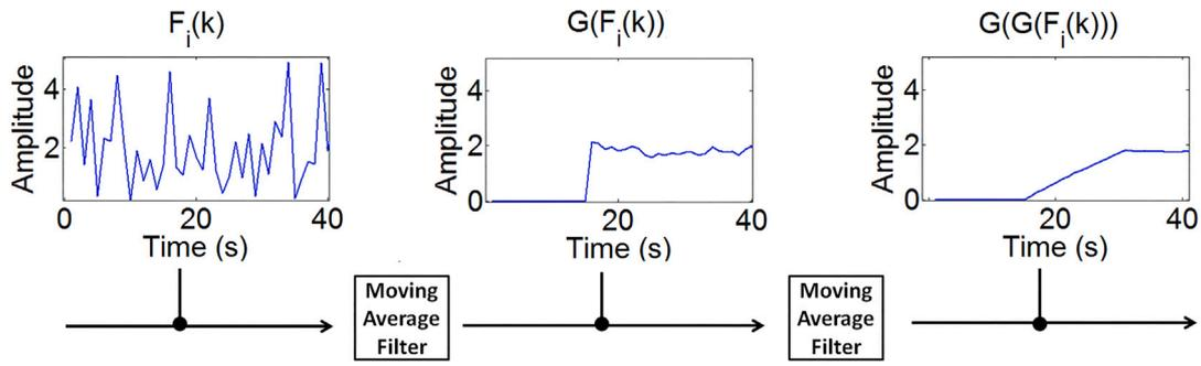
Fig. 11. Delay caused by the Moving Average Filter.
