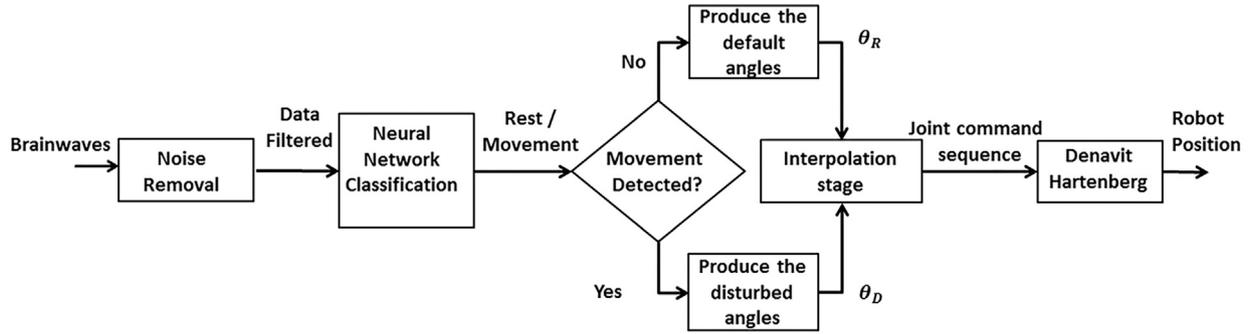
Fig. 7. Translation of brain signal to movement.
