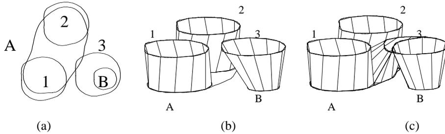
Fig. 1 - (a) Original contours  $\{A,B\}$  (lower level) must be matched against  $\{1,2,3\}$  (upper level). (b) Intuitive match. For simplicity the tiling in polygon A is not shown. (c) Barequet-Sharir match.
