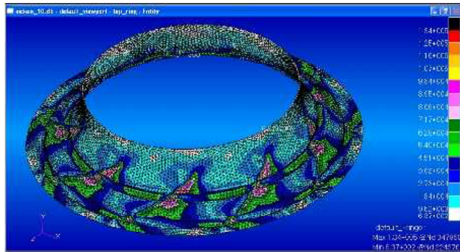
Figure 24: Von Mises stress distribution on the top ring after being beaded.
