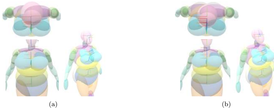
Figure 2.14: Correction of central ellipsoid symmetry of ellipsoids from Tall Chubby. (a) Asymmetric model. (b) Symmetric model.
