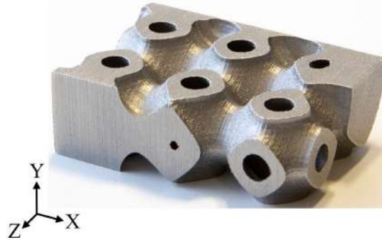
(e) Selective laser melting. View 2.
