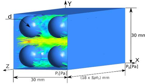
**Fig. 2:** Regular packed sphere case
