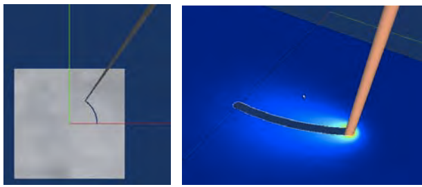
(a) Laser cutting simulator. (b) Cutting simulator integrated with the FEM solution.
