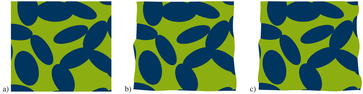
Fig. 2 Stretch mode u_{M1,1} of a micro volume ( l = 4 mm) consisting of stiff particles (blue) in a matrix (green) which is factor f = 0.1 softer, a) Voigt limit (linear displacements), b) minimal boundary conditions and c) Reuss limit (constant tractions).
