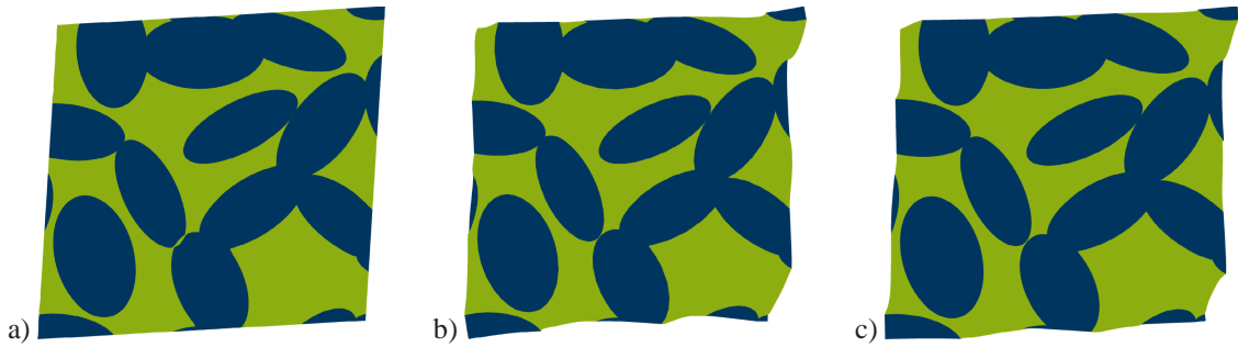
Fig. 3 Symmetric shear mode 1/2(u_{M1,2} + u_{M2,1}) of a micro volume ( l = 4 mm) consisting of stiff particles (blue) in a matrix (green) which is factor f = 0.1 softer, a) Voigt limit (linear displacements), b) minimal boundary conditions and c) Reuss limit (constant tractions).
