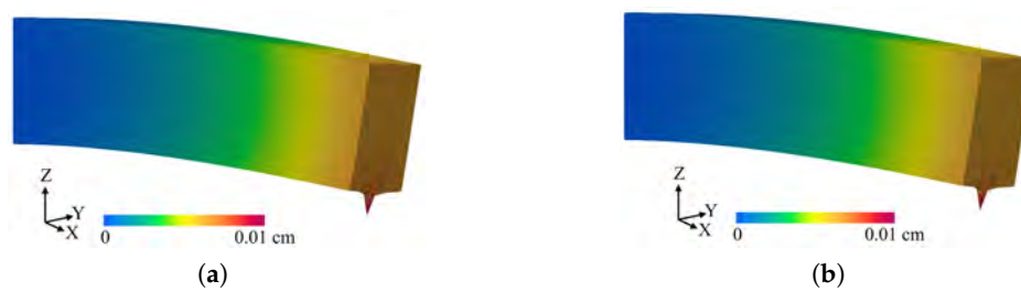
Figure 12. Displacement fields using two Solid Isotropic Material with Penalization (SIMP) modified algorithms. (a) Algorithm SIMP modified to avoid relative density polarization to 0 and 1. Density map in Figure 9b. (b) Algorithm SIMP modified by avoiding relative densities below 0.3. Density map in Figure 11a.
