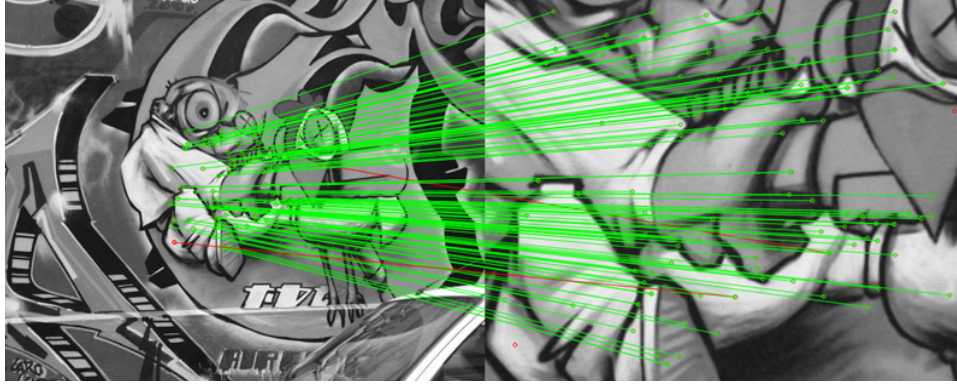
FIGURE 2.2. Correct matches(in green), wrong matches(in red) between two images.
