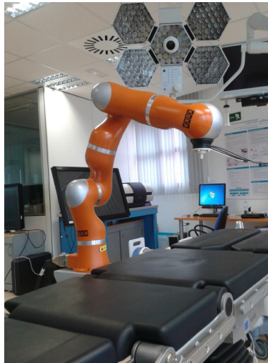
FIGURE 1.7. KUKA LWR IV+ lightweight robot embedded to a surgical bed. Courtesy of Vicomtech-IK4, eHealth and Biomedical applications lab.
