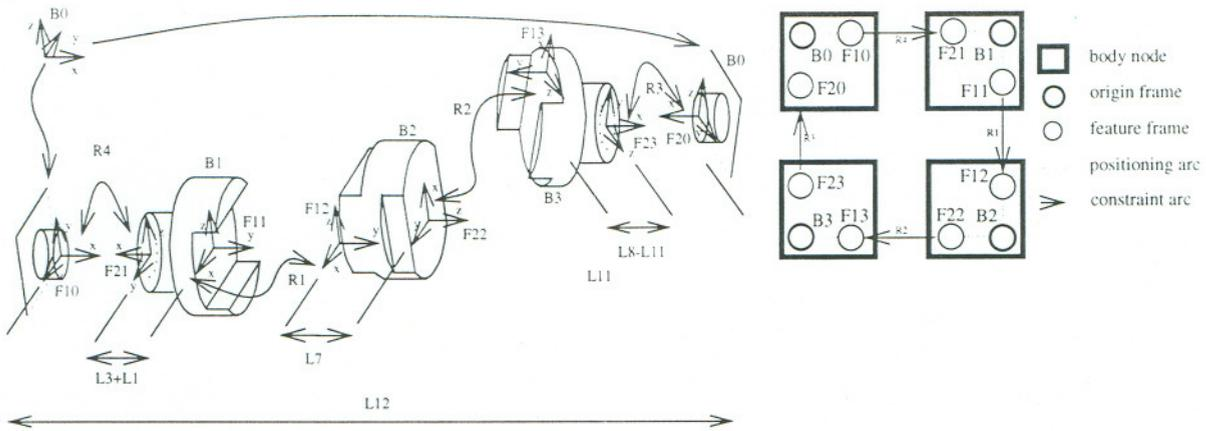
Figure 2: Piece Disassembly and Spatial Constraint Graph of Oldham Mechanism
